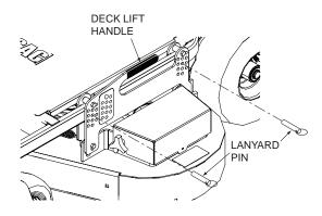
Figure 4-3. Adjusting Cutting Height
